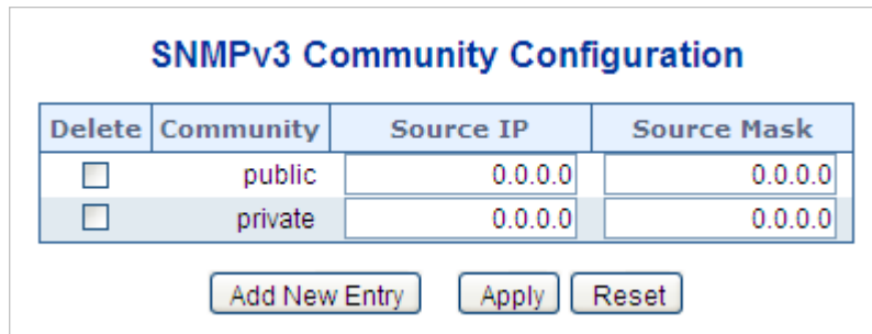
Figure 4-2-2-6: SNMPv3 Communities Configuration Page Screenshot
