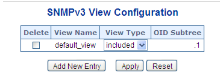
Figure 4-2-2-9: SNMPv3 Views Configuration Page Screenshot
